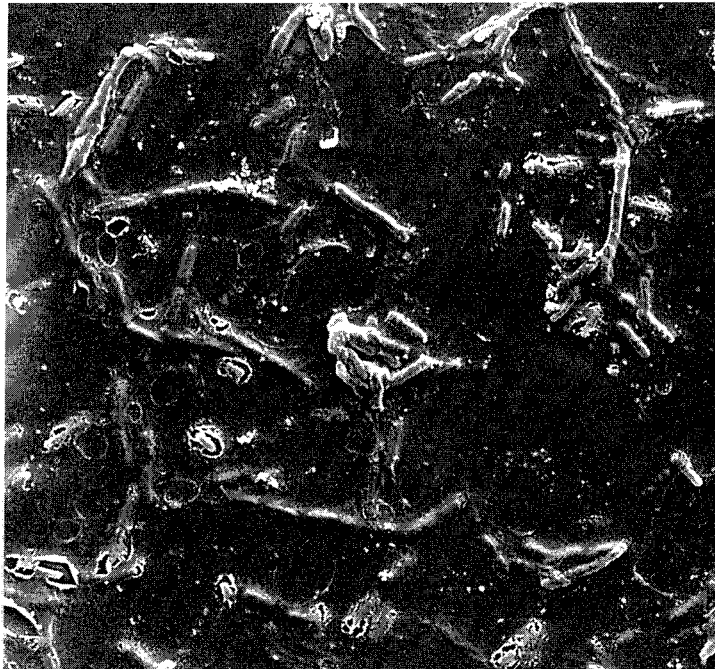
Fig. 3-11 SEM image of a microscope slide exposed for 161 days to flowing groundwater ( 2.8 \times 10^3 \text{ m sec}^{-1} ) from the Stripa borehole V2, 812-820 m. 1.5 cm = 5 \mu\text{m} ; magnification: x3000.
